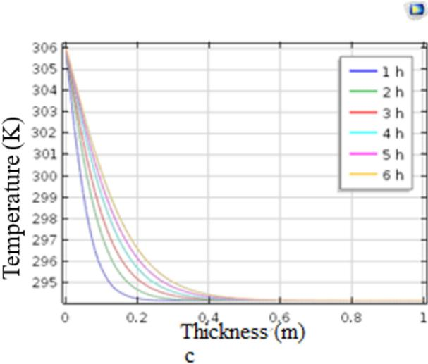
Fig. 4. Temperature profiles through the wall as a function of thickness
