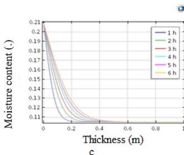
Fig. 5. Moisture content versus thickness profiles across the wall
